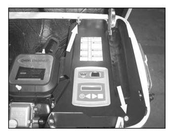
2. Remove controller: Using a Phillips screwdriver remove the four mounting screws from the controller. See Figure 3.
